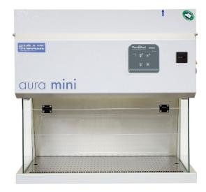
**INWARD** air barrier. In this configuration an air barrier flows through the front opening and is recirculated with the downflow air by a motor blower. 70% of the air is returned to the work area through the main HEPA filter and 30% is exhausted into the environment through a Filtrete® exhaust filter with gravimetric efficiency of 99% on 3µm particles. In this configuration an excellent product protection is ensured, as well as an outstanding containment.
